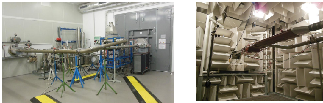
Fig. 9: Acoustics test performed at anechoic chamber with the aircraft air condition component
